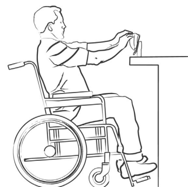
Positioning of counter mounted PED for disabled user
